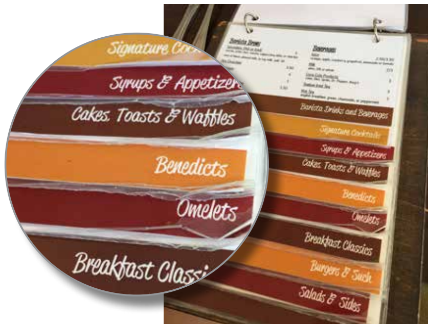
Example of lamination gone wrong
