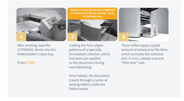
For printers with high volume needs, the stand-alone pressure sealer is an ideal solution. The faster speed, fewer problems and improved visual appeal of the form will yield higher open rates.
